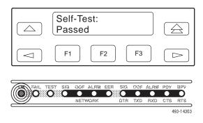
If the self-test fails, the Failed screen appears for five seconds. The Fail LED lights, and an eight-digit failure code (xxxxxxxx) is displayed for use by service personnel to determine the cause of the self-test failure. The DSU/CSU continues to try to operate. If you are in doubt about the results of the self-test, use the Self-Test Health command to display the status of this test (see Self-Test Health in Chapter 4, Maintenance).
